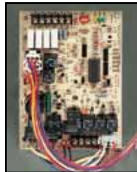
Integrated control board directs gas valve and blower for consistent comfort.
