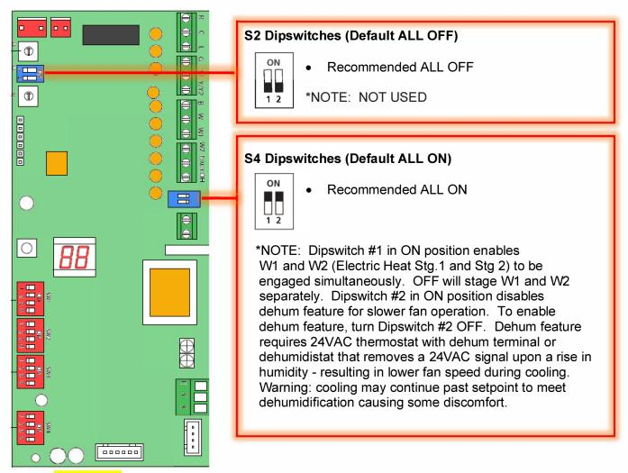
4. SET **OUTDOOR DIPSWITCHES FOR APPLICATION** – Power down before switch adjustments
